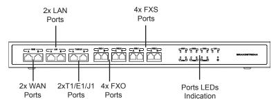
The front panel contains the internal HA100 ports:
